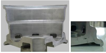
Fig.3 Shrinkage distribution in real cast part
